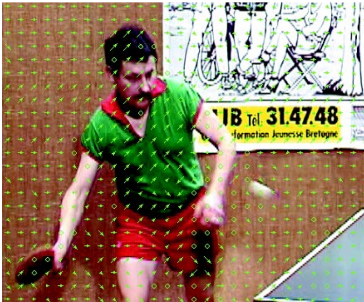
Fig. 5: Display of motion vectors of predicted frames (B and P), overlaid on decoded picture
